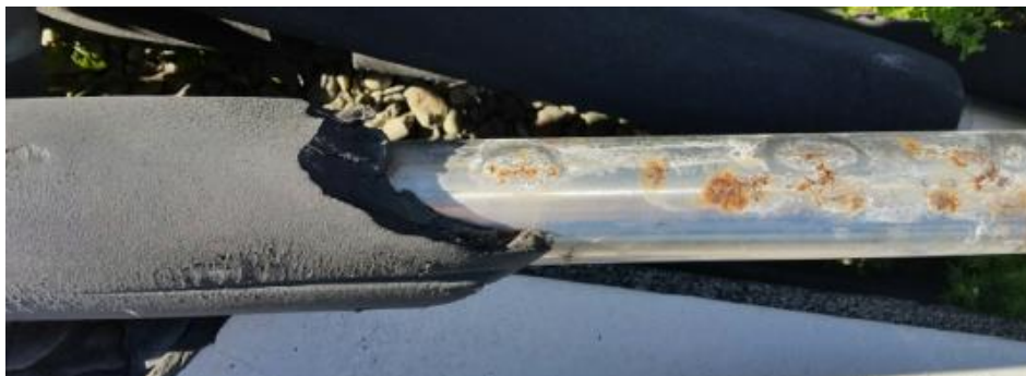
Photo: Venison Processing Plant, NZ – 2015 (SCC and localised corrosion induced by 'standard' lagging).
