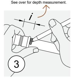
**Mark** the Insertion Depth "*i*" Measure and texta mark the insertion depth (socket depth) from the end of the tube.
