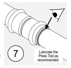
Check the Press Visually inspect the pressed fitting & that the insertion mark is aligned with the end of the socket.
