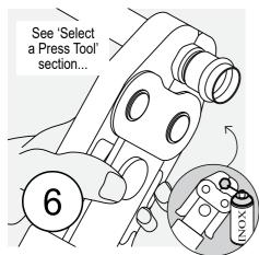
**Press Tool** Selection Use a press tool, jaw or collar to suit the fitting, dimension and application pressures. Ensure press zone is lnox lubricated each press.
