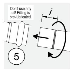
Join the Tube & Fitting Insert the tube into the fitting press socket, turning slightly until it reaches the previously marked insertion depth.
