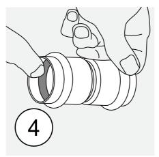
**Inspect** Fitting & Ring Seals Check that the rubber ring seal is not damaged and both fitting & seal are free of debris.
