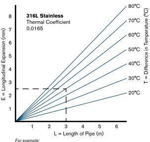
A 3m length pipe at ambient temperature (20°C) is filled with 70°C hot water. The temperature difference of 50°C (70°C minus 20°C) expands the grade 316L stainless longitudinally approximately 2.5mm overall.
