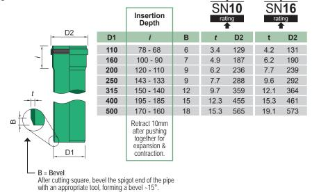
Pipe rated to SN10 is easily identified by green internal surface colour.
