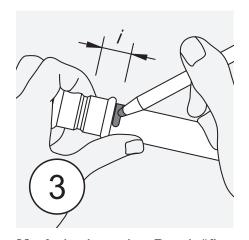
Mark the Insertion Depth "i" Measure and permanent texta mark the insertion depth (socket depth) from the end of the tube.
